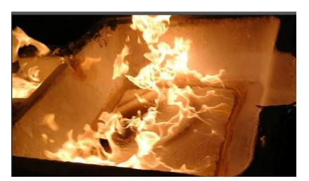
4. Observe change of molten aluminum pressure, control the flowing molten aluminum needed, normal start pressure: 100-150mm, the pressure falls down below 75-100mm when molten aluminum flowing, it will grow later.
