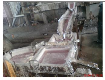
5. Do not shock and beat ceramic foam filter in filtration. Control molten aluminum flow rate in launder.
