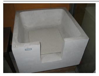
3. Use electric or gas to preheat filter box and ceramic foam filter evenly 15-30 min, make the temperature next to the molten aluminum, ceramic foam filter preheating temperature should surpass 460°C, expansion cotton will seal after heating, it makes ceramic foam filter steady in molten aluminum, preheating makes ceramic foam filter pores open and avoid occlusion expansion and contraction.
