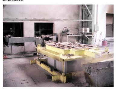
6. Take our ceramic foam filter and clean filter box after filtration.
