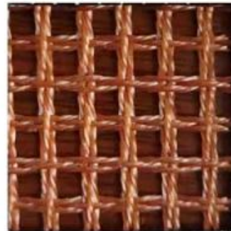
Molten steel filtration
